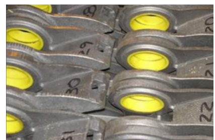
Installed Brake Head Bushings
